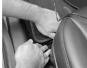
3. Place the N-METER at the appropriate position of the air conditioning vent, and conceal the wires inside the trim panel.
